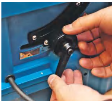
▲ The blade will tilt using the combined tilt and locking knob
